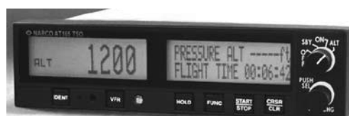
The Narco AT-165 is a modern slide-in replacement for older ARC, King and Narco transponders.
